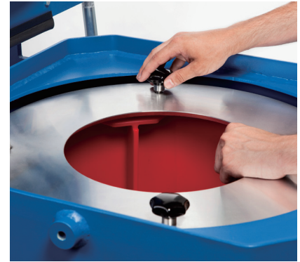
To take the sludge basket out of the drum of a basket centrifuge, four wing bolts must be removed
