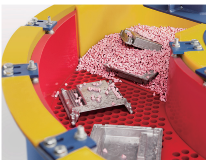
At the exit of the processing channel of the mass-finishing machine, the media and work pieces are separated from each other
